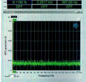
The ADL worked to 192kHz sample rate through its optical S/PDIF input, frequency response reaching 43kHz, our analysis shows, so it well exploits high sample rate. With 24bit PCM, distortion at -60dB was reasonably low, measuring 0.12%, some output amplifier noise influencing this result. Dynamic range was 105dB, good if not up to Astell&Kern's 115dB or so for a portable.
