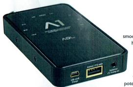
Dominant is the OTG USB port that allows the A1 to be used with a handful of recent Android devices. Thanks to the adjacent mini-USB port, the A1 can act as a computer DAC. The 3.5mm analogue line/ headphone socket doubles as an optical digital output, so the A1 can act as a USB-to-optical converter for high-end DACs.
